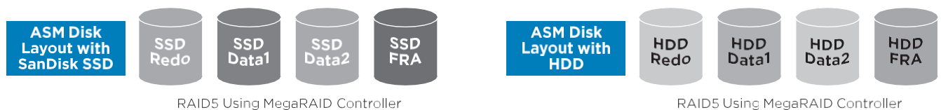
Figure 3: Storage Layout with SanDisk SSD and HDD
